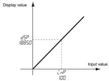
When displaying a flowrate (e.g., in  $\mathscr{U}$ min or  $\mathscr{U}$ h), make the scaling settings after confirming the I/O characteristics of the flowrate sensor. There are flowrate sensors that output analog signals. If this kind of flowrate sensor is used, consider using the K3MA-J.
