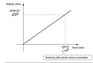
Instead of setting by inputting with the <a> Up Key and <a> Shift Key, current values can be input as scaling input values for teaching. This is useful for making settings while checking the operation status of the K3MA-F.
