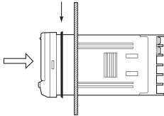
Fit the adaptor into the grooves on the left and right sides of the rear case, then push it until it contacts the panel to secure the K3MA-F.
